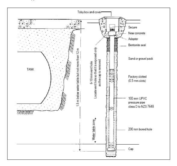
Check observation wells for liquid products using a weighted bailer or a thief pump.
